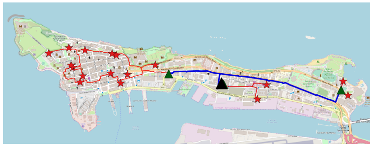
Figure 5-11: Result LV and MV network of reliability model for Old San Juan
